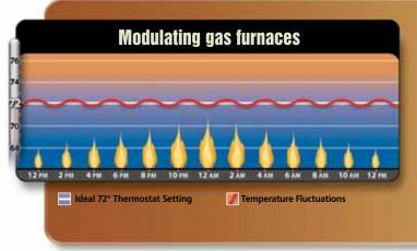
The Coleman® Echelon™ modulating gas furnace has been designed to maintain your ideal temperature by modulating in one-percent increments. Comfort is dramatically increased as the furnace adjusts its level of operation up or down to offset the rate at which heat leaves your home.
