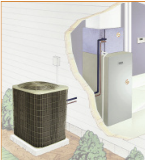
Air Conditioner and Gas Furnace System
